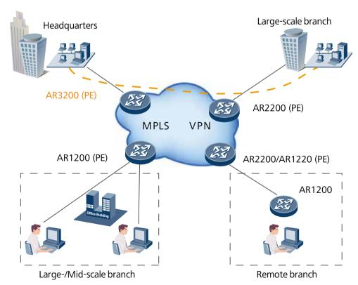
The AR3200 routers are well suited to serve as PEs in the headquarters office of a large enterprise. The MPLS L3 VPN segregates services by type. The AR3200 routers feature flexible deployment, fast distribution, and secure transmission of VPN services, as well as supporting enterprise service operation over networks.
