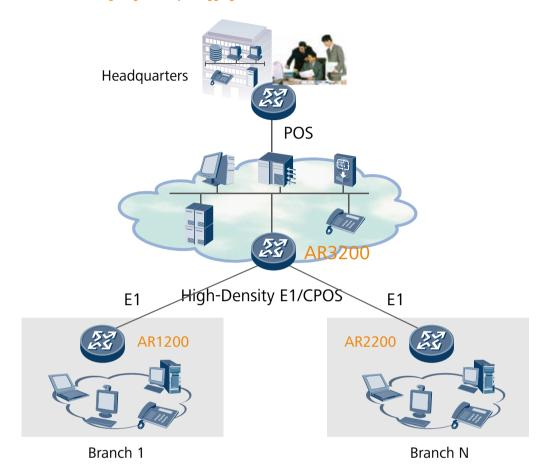
AR3200 series enterprise routers support the rich interface cards, including high-density E1, CPOS, POS interface cards and so on, to meet the convergence access requirements in the various branches and headquarters. Multiple enterprise small branches connected by E1 uplink to the aggregation layer routers. The aggregation routers use high-density the E1 boards or CPOS to converged access, and then through the POS uplink to connect the high-end router of the core network.
