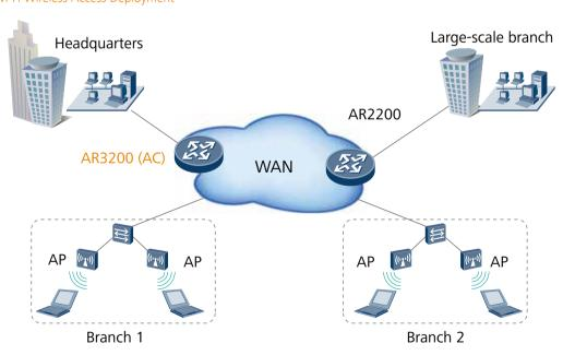
The AR3200 routers integrate AC (Access Controller) functionality, which can manage the wireless AP (Access Point) in wireless LAN. AR2200 supports rich certification and flexible user access control, which can provide security access guarantee for Wi-Fi users. The rich wireless capabilities integrated in one device, this can realize centralized management of wired and wireless networks, to meet the requirements of different scale enterprises networks.
