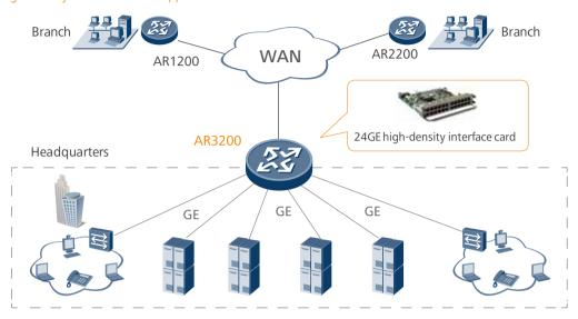
To preserve customer investment, the AR3260 features a highly modular design. In the example above, a high-density GE access interface card is deployed to provide Gigabit speed access for servers and workgroups at enterprise headquarters.
