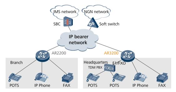
The AR3200 routers integrate voice, fax, and IP services. For enterprise users, the AR3200 routers serve as a SIP access gateway for the headquarters office, transforming phone signals into VoIP signals. The AR3200 routers uplink interfaces connect to the IP Multimedia Subsystem (IMS) or Next Generation Network (NGN) to allow any media, including phones, handsets, and computers, to communicate at any time.
